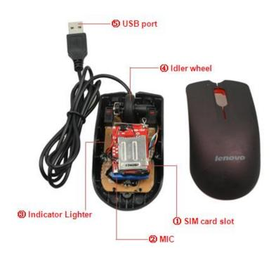
1. SIM card slot 2. MIC 3. Indicator Lighter 4. Idler Wheel 5. USB port
